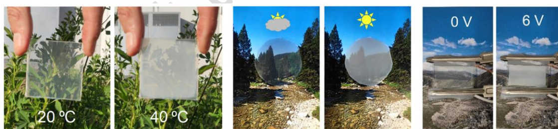
Figure. Transparent-to-opaque transitions achieved in our SW materials upon temperature variation, sunlight illumination and application of external voltages.
